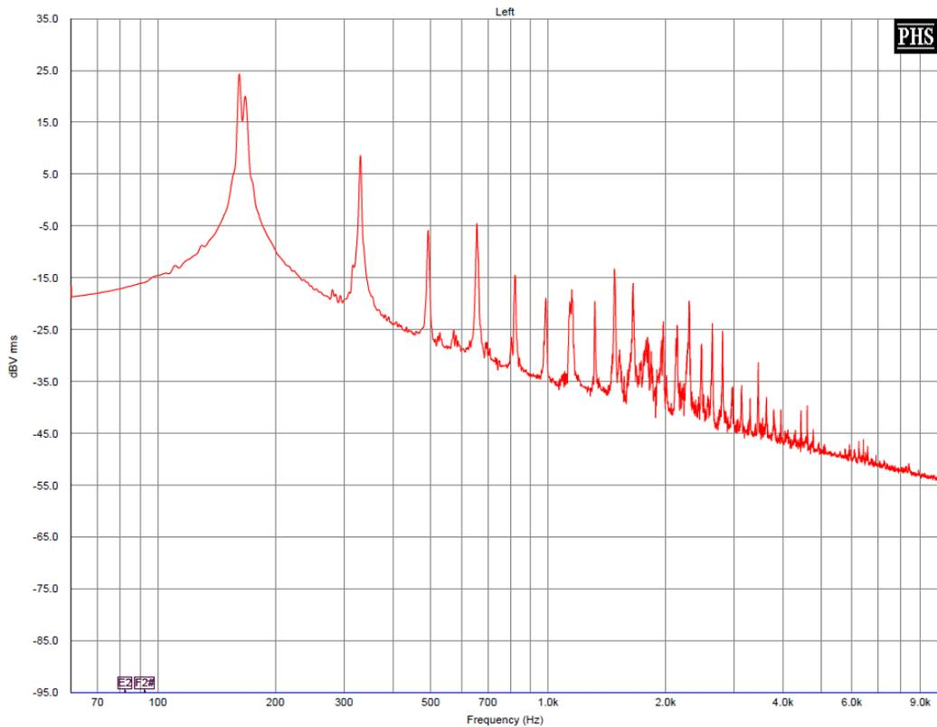
Figure 1 The red line is the Amplitude –Frequency spectrum of a “wolf note”. The fundamental frequency (left most peak) has a double peak which creates a beating sound. The other peaks are at frequencies that are exact multiples of the fundamental.
