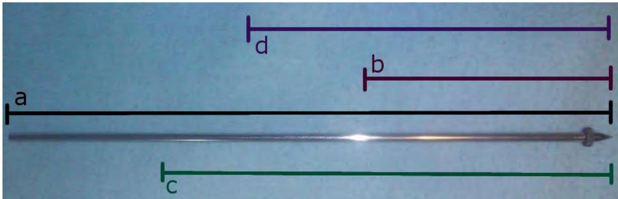
**Figure 1 a) total length, b) cellist's clamp point length, c) resonant point length, d) length to cut endpin.**
