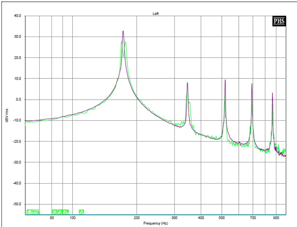
Figure 2 Amplitude- Frequency graph of a cello playing the "wolf note", green, and then the same note on the same cello with the endpin on a CelloStone, purple.
